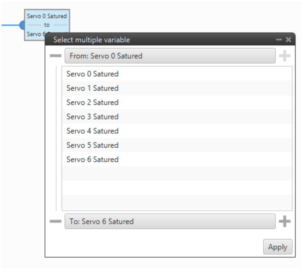
4. A **PWM block** to indicate the PWM variables to which the PWM pulse should be transmitted for each servo.
