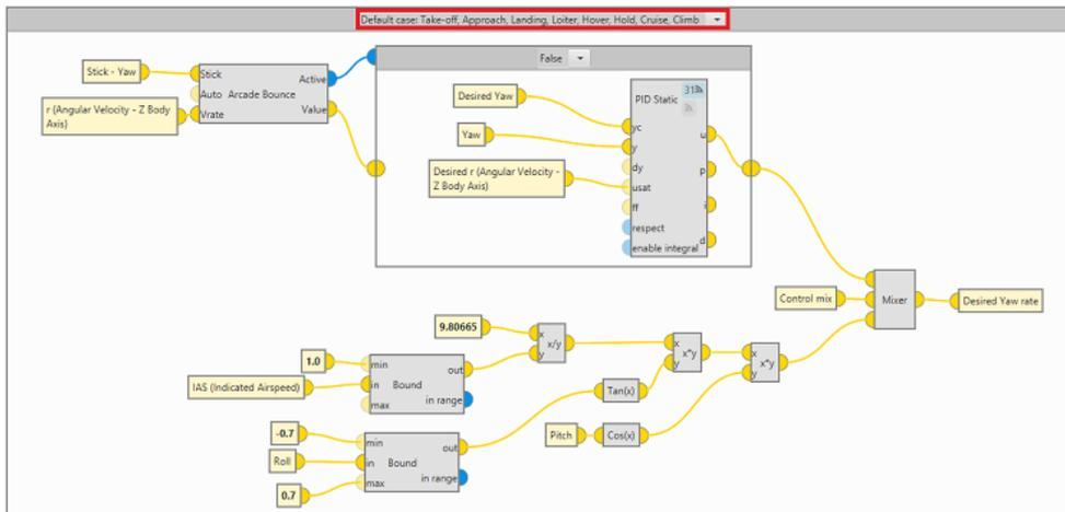
The program logic has been divided into three sections/parts. Two of them to define the aircraft control according to the flight configuration and, once these controls are defined, in the third section of this program, the output signals of both are provided to the Control mix variable by means of the **Mixer** block.
