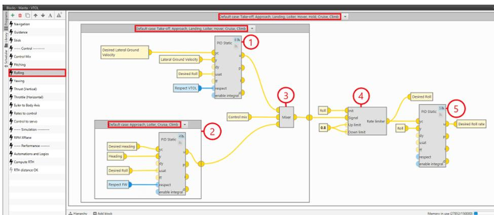
The program is basically controlled by 3 PID controllers, which provide the speed ratio as a function of the input variable and the desired variable.
