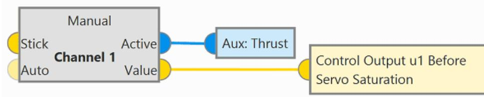
The Value output of this block must be linked to the Control Output u1 Before Servo Saturation variable, since this variable controls the actuation of the Thrust defined in the **Actuator** block.
