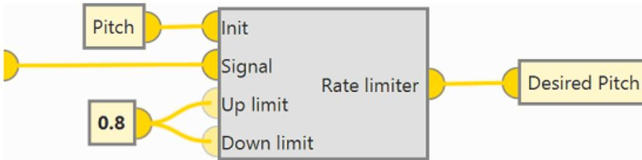
The Signal input variable of the **Rate limiter block**, Desired Pitch, is generated by the **Guidance program**. In the Hold flight phase it is intended to stabilize the aircraft attitude, that is why the Desired Pitch control is independent of the flight configuration.
