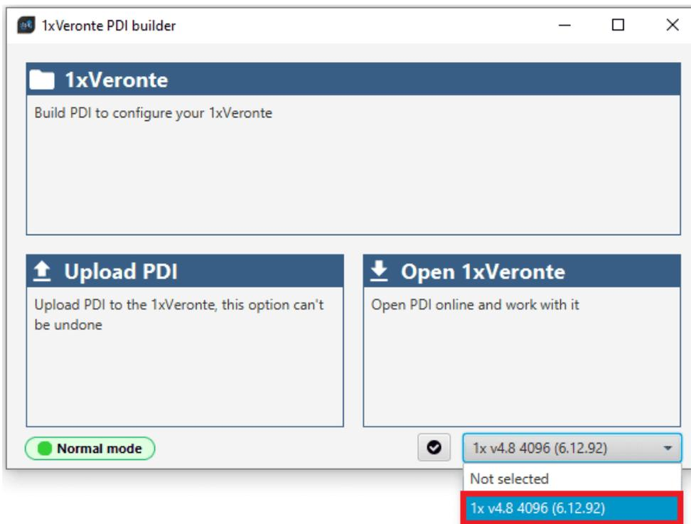
2. Select the **Open 1xVeronte** option to directly edit the configuration loaded in the 1x:
