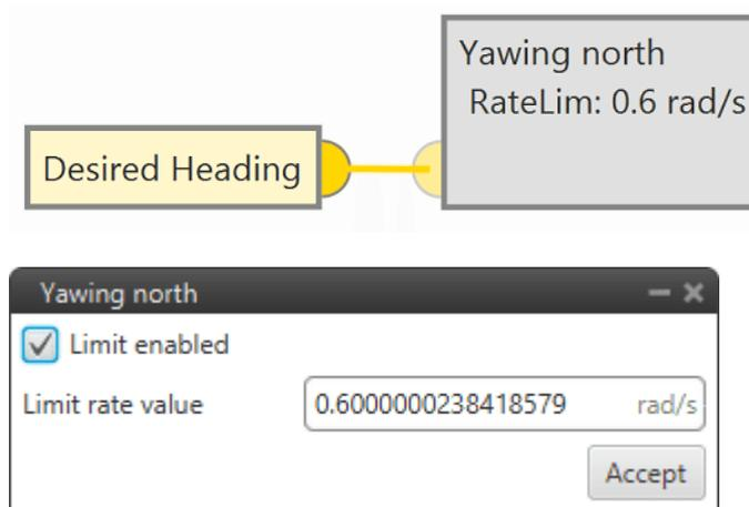
In this case, the variable Desired Heading is connected to the input, so Desired Yaw = Desired Heading.
