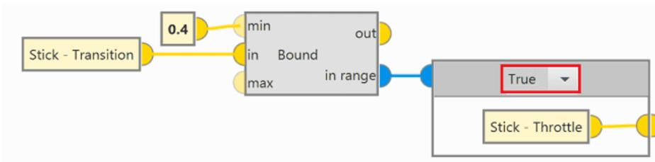
Otherwise, if this variable has a value **less than 0.4**  $\Rightarrow$  in range bit will be **false** and the Stick input will have a value of **0.0**.
