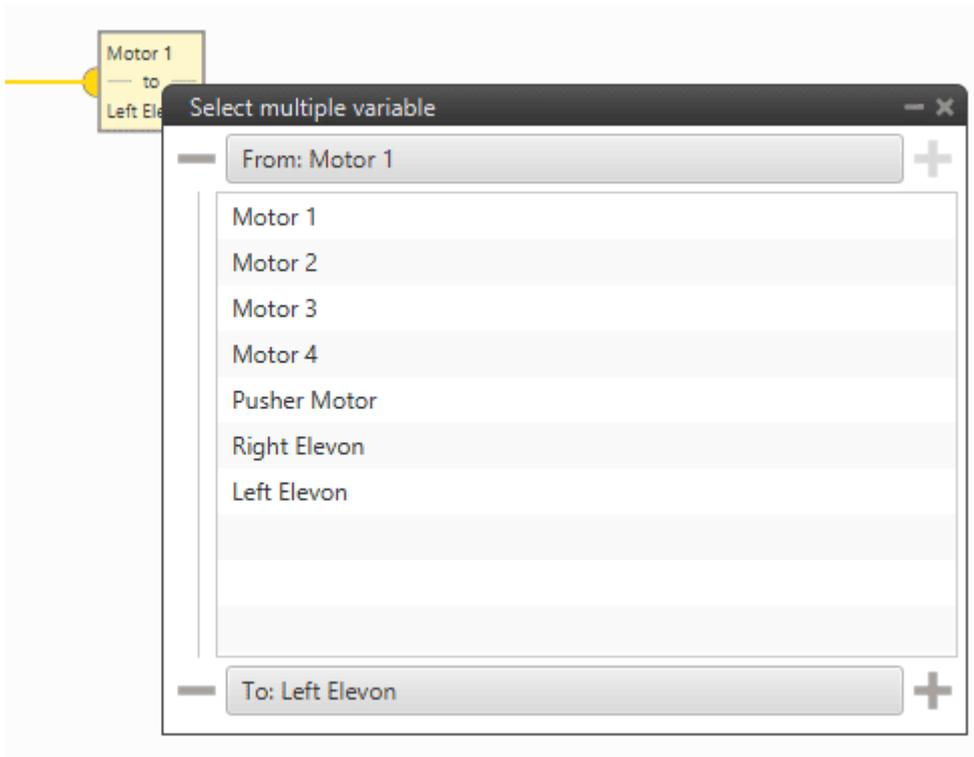
6. A [Write multiple Reals block](#) with the variables for Control actions after servo saturation.
