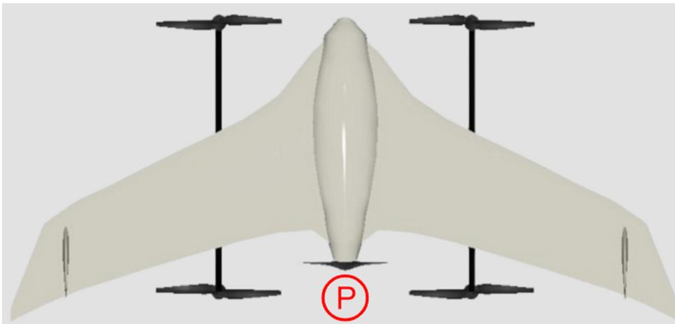
Throttle actuation is performed with the use of **Channel 5**. This channel is controlled with the **Manual** block, which is configured to process throttle control depending on the control mode. This block switches between two input signals according to the current mode of the configured channel.
