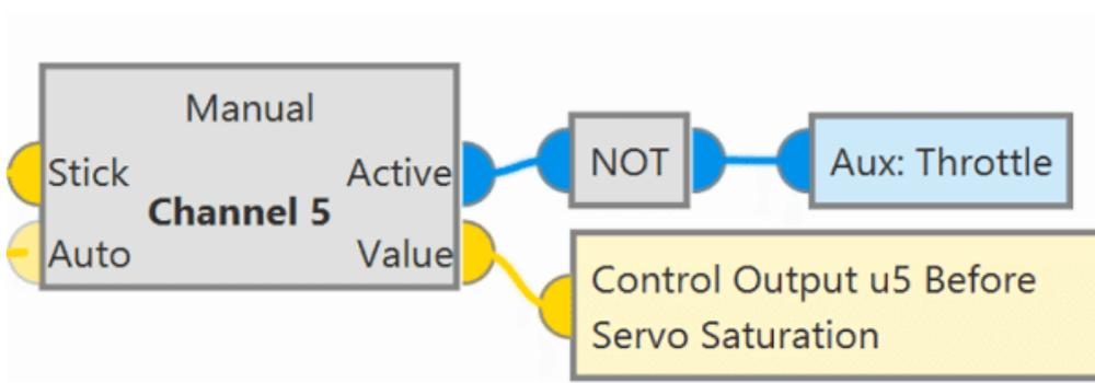
The Value output of this block must be linked to the Control Output u5 Before Servo Saturation variable, since this variable controls the actuation of the Throttle defined in the [Actuator block](#).
