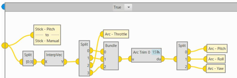
The behavior of this block depends on the value of the output Status of the Stick block. When this output is **True**, the output Y data of the Stick block is linked to this block as an entry and the transformation of the values of this output follows the following logic:
