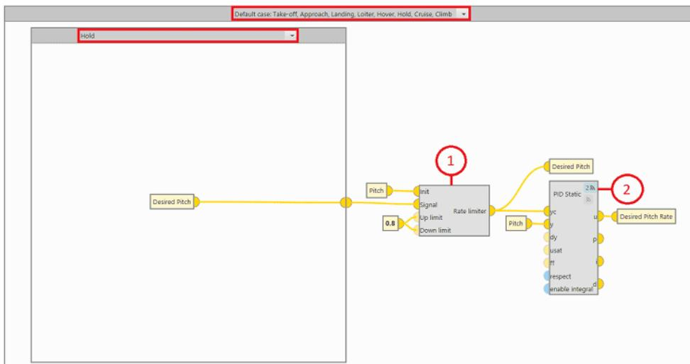
1. The **Rate limiter** block is defined to adjust the input signal to a controlled gain.
