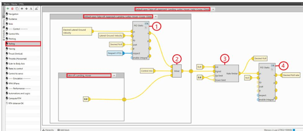
In these flight phases the **FW** flight configuration is not taken into account, since **these flight phases must be performed in quadcopter configuration**. For this reason, **no PID** controller is defined to control the **Heading**.
