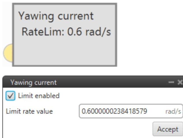
With the Yawing current block it is intended that the aircraft **maintains the yaw angle it has when entering the phase**, i.e. Desired Yaw = Current Yaw.
