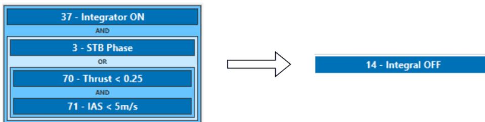
When **Integral OFF** is triggered, a value of **0** is stored in the Integral Enable bit, turning **false**. Therefore, the enable integral input of the PDI controller is false, which implies that the integral term is exponentially discharged.
