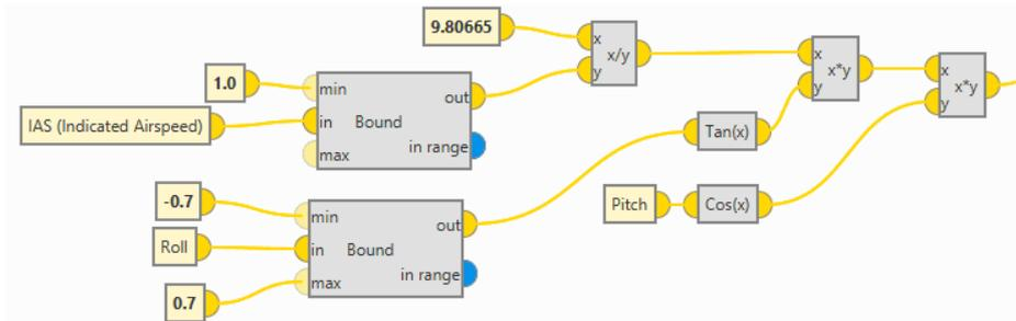
**Bound** block limits the **IAS** and **Roll** values. The minimum value for the **IAS** is 1.0 *m/s* , and the value for the **Roll** angle should be between  $[-0.7, 0.7]$  *rad* .
