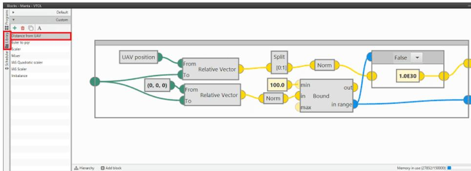
The distance **from the UAV position to the predefined point** and the distance **from the NED origin to the predefined point** are calculated. These distances are calculated using the **Relative Vector** block, which returns a relative vector in NED frame from the two input positions. For more information on this block, visit the [Positions blocks - Block Programs](#) section of the **1x PDI Builder** user manual.
