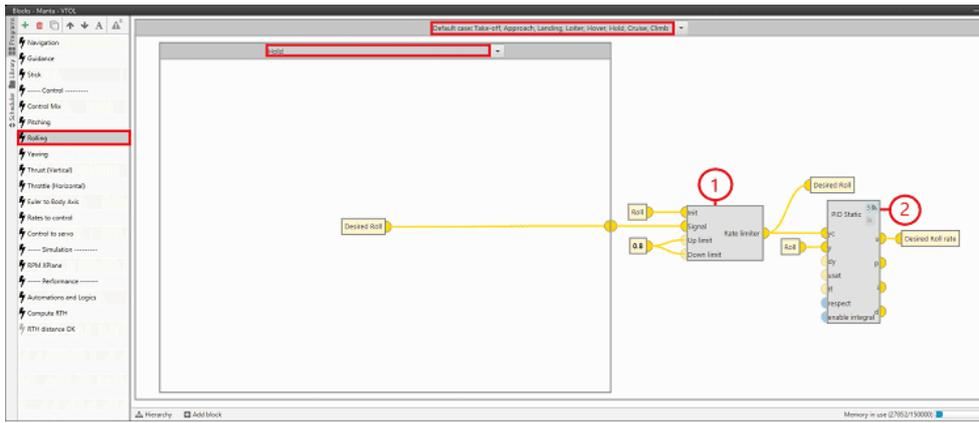
In this flight phase it is **not necessary** to define the **Roll control**, since it is intended to keep a **constant attitude** of the aircraft, so the value of the **Desired Roll** variable will come directly from the [Guidance program](#).
